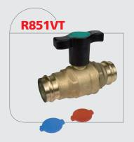
Brass-finished ball valve, press-fittings with black O-ring according to standard EN681-1 for water distribution plants (drinking and heating water) and with extended plastic T handle for pipes with high insulating thickness. Full port. W Series.
