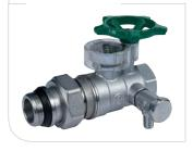
Chrome plated ball valve, female-male connections with pipe union and slowed down operation and 1/4" drain tap.
