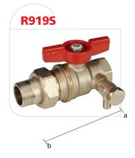
DADO® ball valve, nickel plated, female-male connections with pipe union, red T handle and drain tap. Full port.
