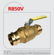
Brass-finished ball valve, press-fittings with yellow O-ring according to standards EN549 and EN682 for gas and hydrocarbon fluids distribution plants and yellow lever handle. Full port.
