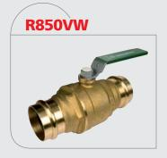
Brass-finished ball valve, press-fittings with black O-ring according to standard EN681-1 for water distribution plants (drinking and heating water) and green lever handle. Full port. W Series.
