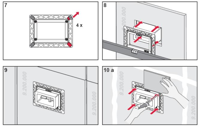
7. Peel off the sticker 8. Place it on the gyps sheet. 9, Stick it on the gyps sheet. 10 a. Take the marbel or tile you wish to fix. And unscrew the inner plate matching with the thickness normally 5 to 18 mm.
