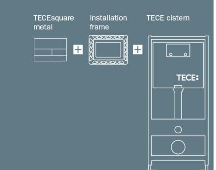
1 > Flush mounted plates are applicable for TECE square metal by default.
